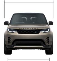
Front wheel track Air suspension 1.692,4mm
